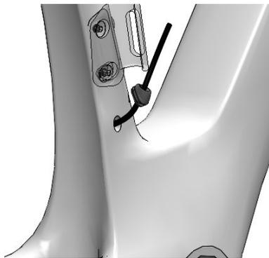
Route the front derailleur Di2 cable through the seat tube hole to the bottom bracket exit port.
